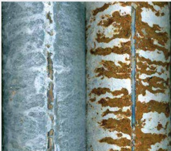
Magnelis® ZM120 welded, not re-protected
