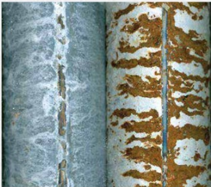
Magnelis® ZM310 welded and re-protected
